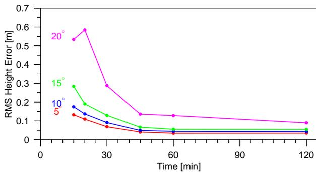
Fig. 11. RMS of height errors for varying batch lengths, with estimated residual tropospheric zenith delay and a constant weighting function.
