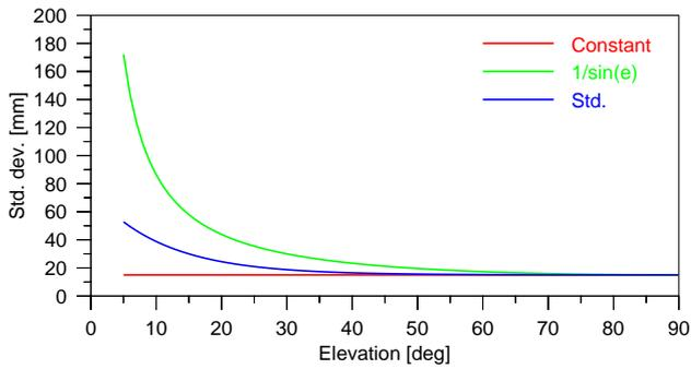
Fig. 4. Functions that map the a priori precision of the phase observations as functions of satellite elevation.
