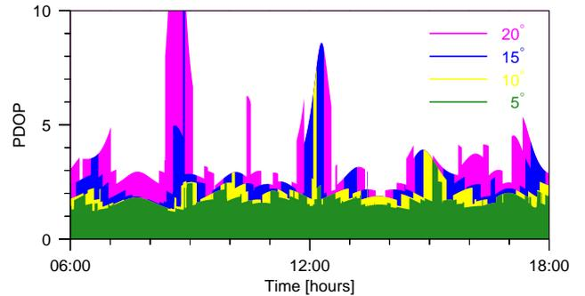
Fig. 5. PDOP using different elevation cutoff angles. Peak values (outside plot range) reach approx. 14 for 15° cutoff and approx. 23 for 20° cutoff.
