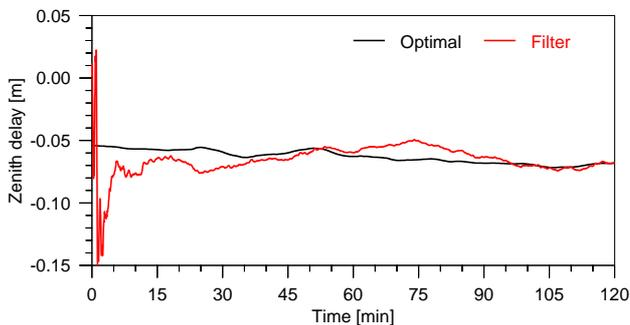
**Fig. 7.** Estimated residual tropospheric zenith delay. Both solutions are computed using the standard stochastic model and  $5^\circ$  elevation cutoff angle.
