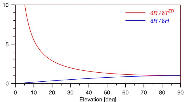
**Fig. 1.** Partial derivatives of the observed range with respect to tropospheric zenith delay and station height respectively.
