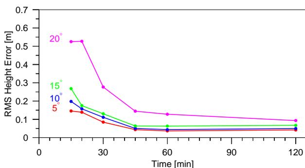
Fig. 13. RMS of height errors for varying batch lengths, with estimated residual tropospheric zenith delay and the reciprocal of sine as weighting function.
