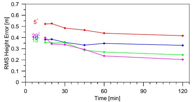
**Fig. 9.** RMS of height errors for varying batch lengths, using the a priori troposphere model only and the standard weighting function.
