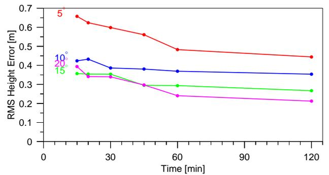
**Fig. 8.** RMS of height errors for varying batch lengths, using the a priori troposphere model only and a constant constant weighting function.
