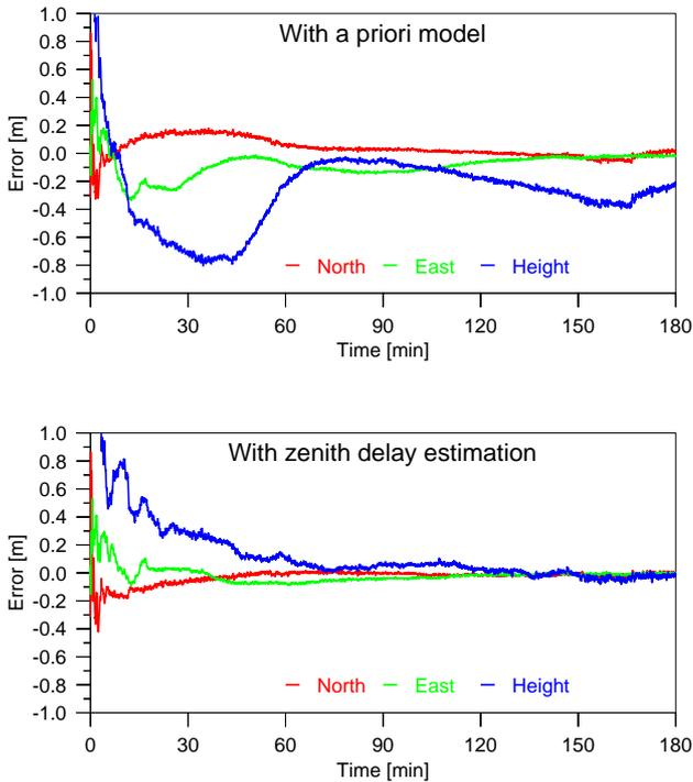
**Fig. 6.** Position errors with a priori troposphere model only (*top*) and with estimation of residual zenith delay (*bottom*). Both plots show the filter solution (no smoothing applied) using the standard stochastic model and  $10^\circ$  elevation cutoff angle.
