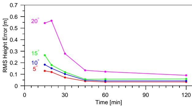
Fig. 12. RMS of height errors for varying batch lengths, with estimated residual tropospheric zenith delay and the standard weighting function.
