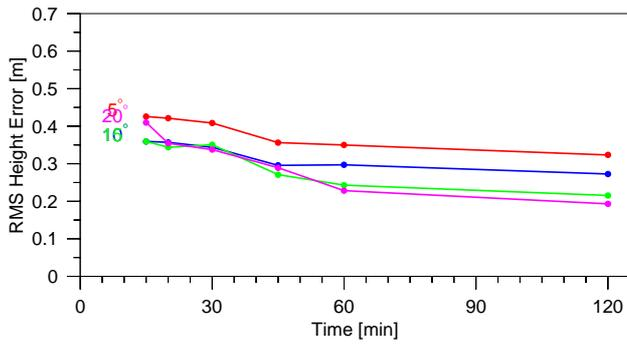
Fig. 10. RMS of height errors for varying batch lengths, using the a priori troposphere model only and the reciprocal of sine as weighting function.
