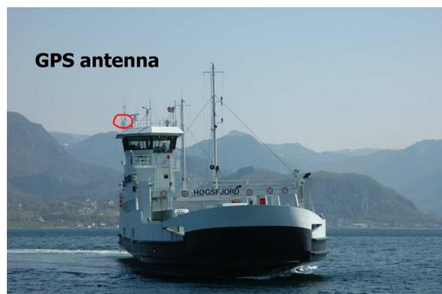
**Fig. 3.** The shuttle ferry carrying the GPS receiver. The location of the antenna is marked with a red circle.
